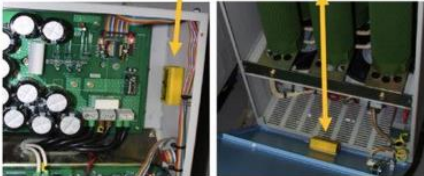
VCI EMITTERS IN ELECTRICAL CONTROL PANELS
