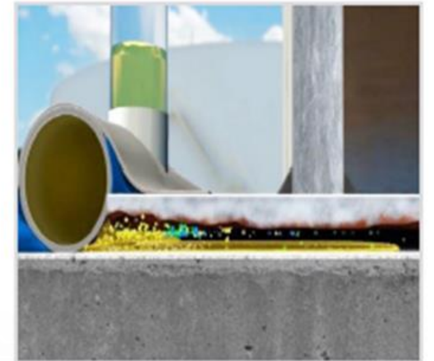
VCI Dispersion from Slurry
