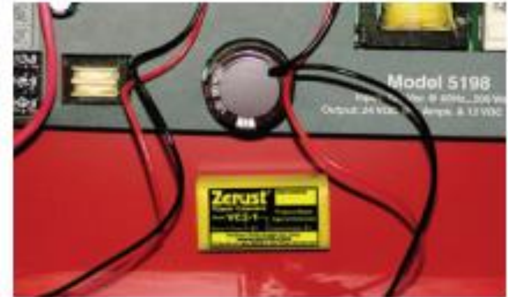
Zerust VC2-1 Vapor Capsule protecting energized electrical connections in a small enclosure.
